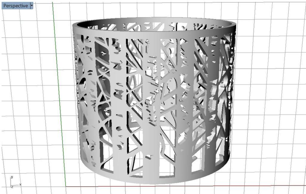
**Figure 1.4** extruded polysurface flowed to the original surface.
